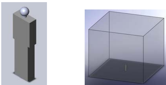
Fig. 2 Human body model Fig. 3 Calculation region schematic diagram
